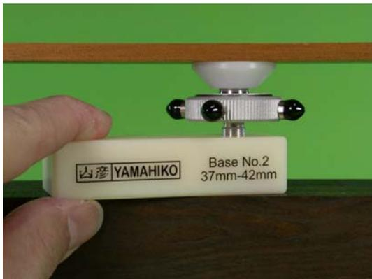
Turn **the sensor** left for *more 90 degrees* (remember that four **output connectors** are ready in every 90 degrees) to push up **the contact chip** onto the soundboard more tightly and stably.
