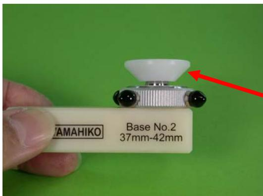
And **Contact chip** is installed.
