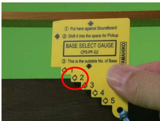
As shown in the left picture, the **base select gauge** will find the suitable No. of the base.
