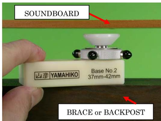
Then turn **the sensor** part left to pull it up until the **contact tip** *lightly* touches the soundboard and stop it. Remember which **output connector** (any one out of four) faces in approximately best direction for cable connection.
