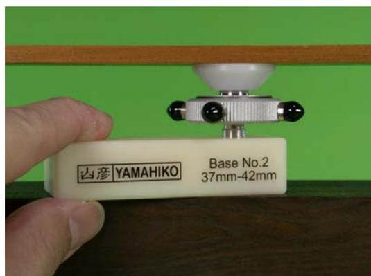
Turn **the sensor** left for *more 90 degrees* (remember that four **output connectors** are ready in every 90 degrees) to push up **the contact tip** onto the soundboard more tightly and stably.
