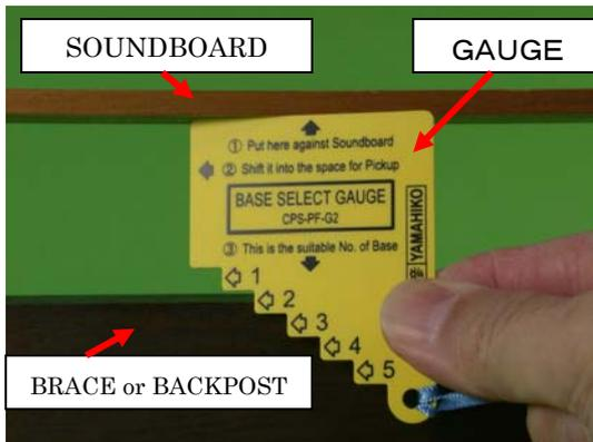
First of all, measure the space between soundboard and brace/backpost to select **the base** part with most suitable thickness. The yellow “**base select gauge**” will indicate the best fit **base** when you insert it between the sound board and brace or backpost.
