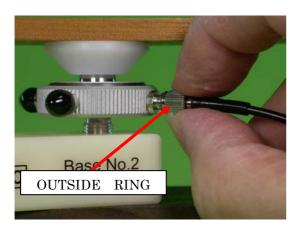
Screw the outside ring of the **output cable** to fix it to the **output connector** of the **sensor**.
