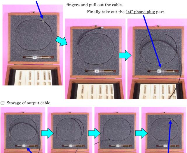
At first, insert the 1/4 phone plug into the cushion and snap the cables into the grooves of the cushion in sequence as shown in the picture.
