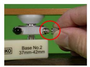
Then turn **the sensor** part left to pull it up until the **contact chip** *lightly* touches the soundboard and stop it. Remember which **output connector** (any one out of four) faces in approximately best direction for cable connection.
