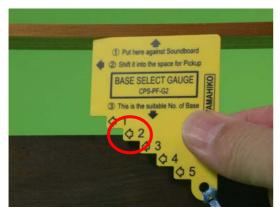
As shown in the left picture, the **base select gauge** will find the suitable No. of the base. In the left case, the **gauge** stops in No.2, the **base**
