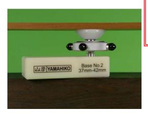
Base No.2 37mm-42mm Then turn **the sensor** part left to pull it up until the **contact tip** *lightly* touches the soundboard and stop it. Remember which **output connector** (any one out of four) faces in approximately best direction for cable connection.
