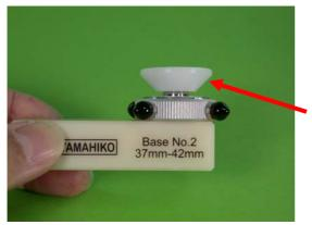
Then put **the sensor** into the selected **base**, screwing it into the hole of the **base** until the bottom part of **the sensor** touches on the surface of **the base**.
